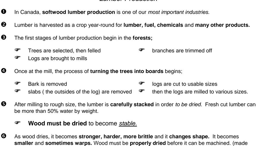
Wood can be Air-dried (left outside protected from the elements) or Kiln-dried (heated in a
