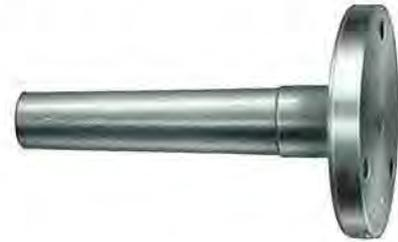
The advantage of it will be quickly seen where it is necessary to turn small pieces which cannot be held between the conical centres. The centre of the plate is drilled to take an ordinary wood screw, which is operated through a hole in shank, while additional holes are drilled in the plate for securing the work. It is provided with a No. 2 Morse taper shank to fit into the driving headstock. Two sizes are available with driving plate diameters of  $2\frac{1}{4}$ " and  $3\frac{1}{4}$ ".
