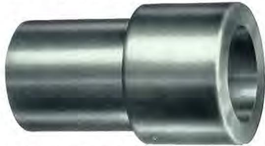
This is very useful as a quick acting chuck. It is bored with a taper hole to hold the work firmly and is screwed internally to fit the headstock spindle. The sizes given indicate the diameter of the hole to receive the work. 1", 1½", 2", 2½".
