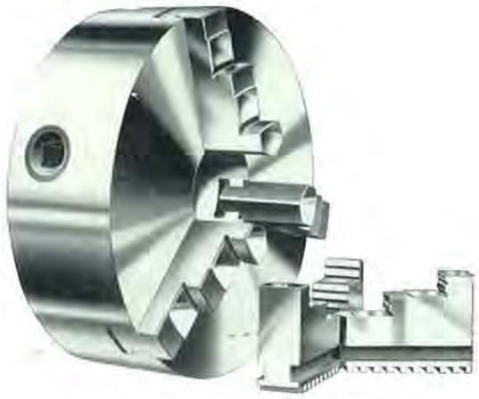
Where aluminium or similar light non-ferrous parts are to be handled this chuck is provided. It is suitable also for holding such articles as wood bowls, etc.
