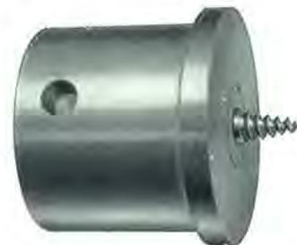
This chuck is for rapidly centring small work, which is held by the taper screw. The further the work is screwed in the tighter it is held. The chuck is screwed internally to fit the headstock spindle. Two sizes 3" and 4" diameter.
