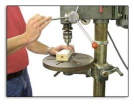
2. Lay the car blank on its side and drill the axle holes. Axle holes should be drilled perpendicular to the car's longitudinal axis in order for the car to roll freely and straight down the track. A drill press is highly recommended because it makes drilling perpendicular holes a cinch.
