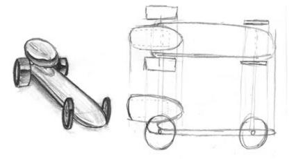
design. Show the location of hidden details (such as the cartridge hole) by using dashed lines.
