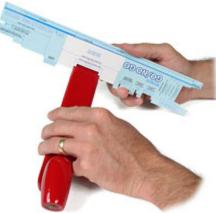
Vehicle weight is a critical factor in competition. Because weight is an enemy of speed, the idea is to get the weight to the absolute minimum. Remember to weigh the car with all the wheels and hardware (axles, washers, screw eyes, and so forth).
