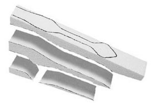
3. Smooth the corners of your prototype with a sharp knife, the hot wire cutter, or sandpaper. **Note:** You may have limited success with sandpaper on polystyrene.
