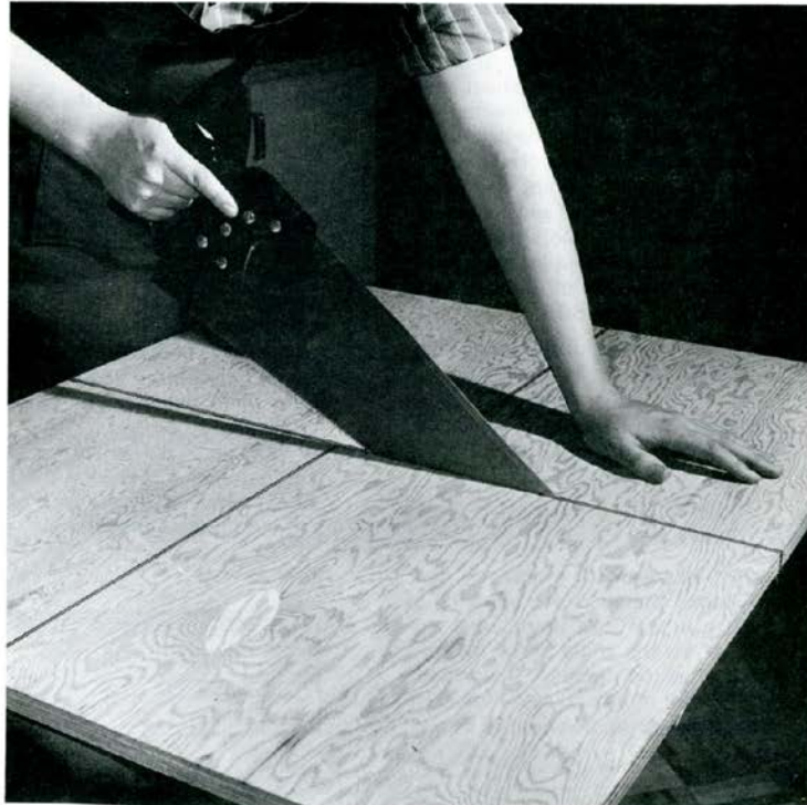
Fig. 8:13 Use double layout lines when cutting plywood.
